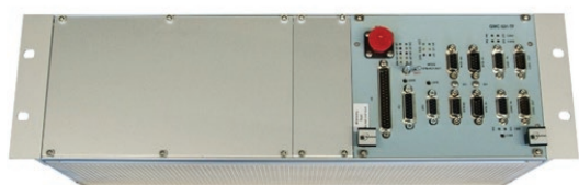
Fig. 1 WAG DIAGNOSTIC on-board diagnostics system – WTB gateway and integrated system block
