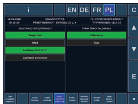
Fig. 2 UIC 557 compliant user interface
